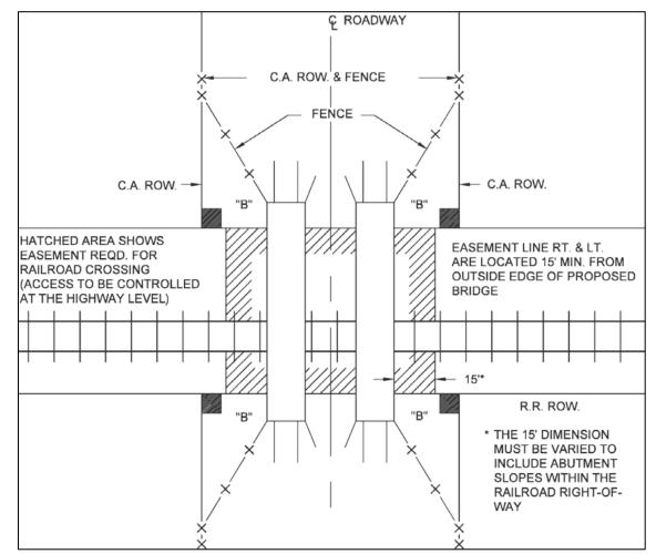
Figure 1-8 indicates a method of showing the easement for a roadway bridge crossing over railroad.
