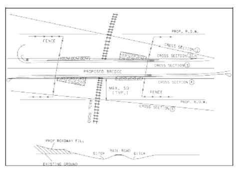
Figure 1-7 Example Cross Section Locations
